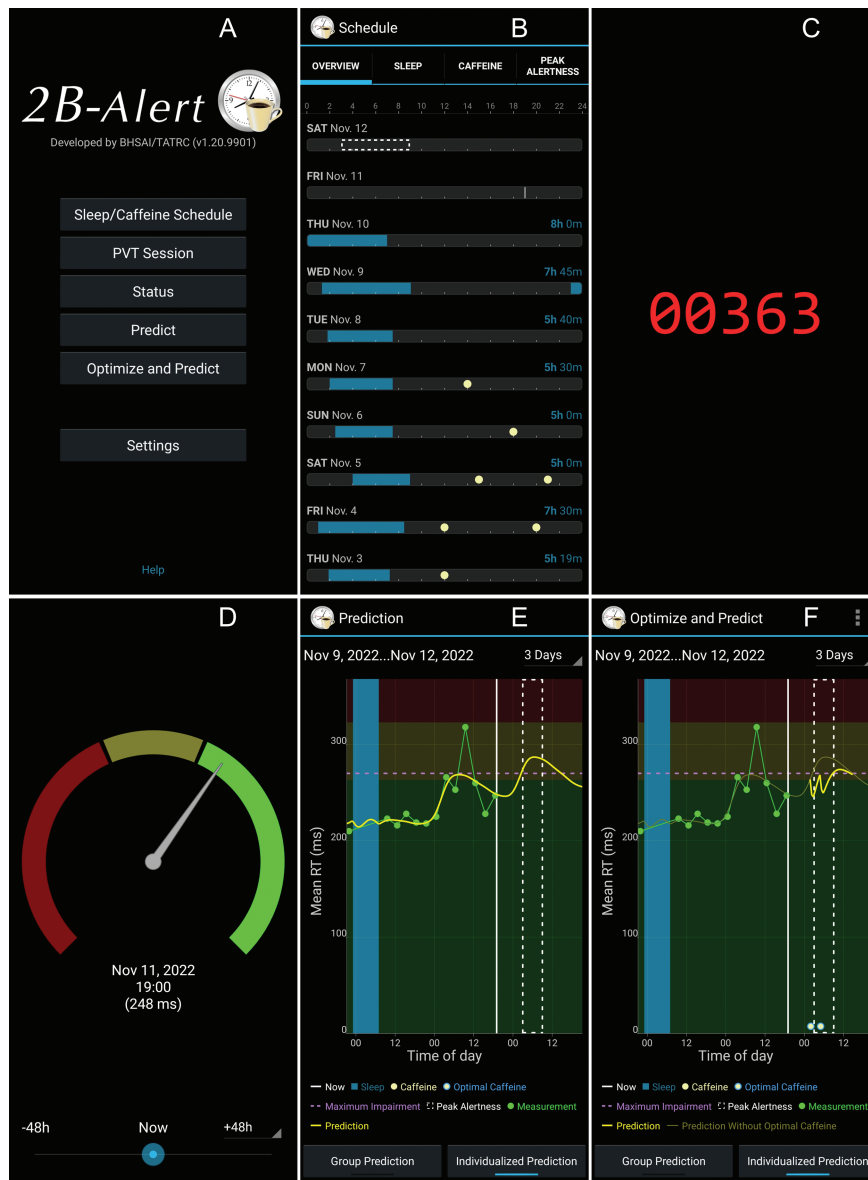
Figure 1. Screen capture of the key components of the 2B-Alert app. (A) The main menu provides access to the app functionalities. (B) “Sleep/Caffeine Schedule” provides an overview of the user’s schedule, showing sleep (blue bars) and caffeine (yellow dots) inputs, as well as the desired period of peak alertness (white dashed box). (C) “PVT Session” allows the user to perform a psychomotor vigilance test (PVT). The image shows a stimulus displayed during a PVT session. (D) “Status” displays alertness predictions through a dial-and-needle representation and (E) “Predict” displays alertness predictions (yellow line) for an individual, or a group of individuals, and the PVT results in terms of mean response time (RT) (green dots). (F) “Optimize and Predict” displays alertness predictions with the optimal caffeine recommendation (thick yellow line) and without caffeine (thin yellow line) and the timing of the caffeine doses (yellow dots with blue circles).
